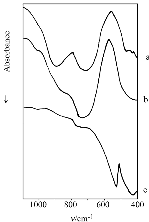
Fig. 5. IR spectra of (a) residue at 350^\circ\text{C} , (b) residue at 550^\circ\text{C} , (c) residue at 1000^\circ\text{C}
